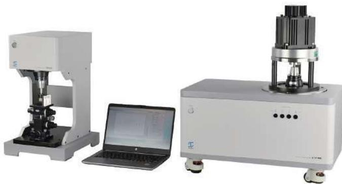
To reduce motor noise and vibration, cogging torque must be measured and reduced. Sugawara's Cogging Torque and Torque Ripple Test Systems can measure cogging torque with high accuracy and no mechanical loss for a variety of motors (DC, DC brushless, AC servo, stepping, etc.). These systems can play a significant role in motor development and quality management.
